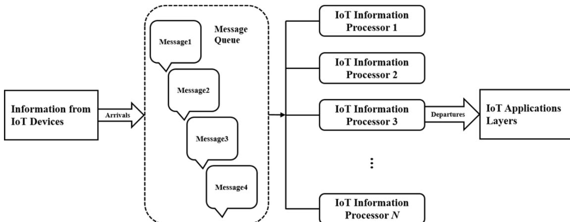
FIGURE 1. Architecture of IoT Message Queue
