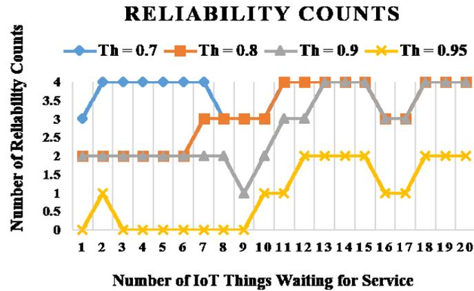
FIGURE 3. Reliability Counts for Variable Threshold
